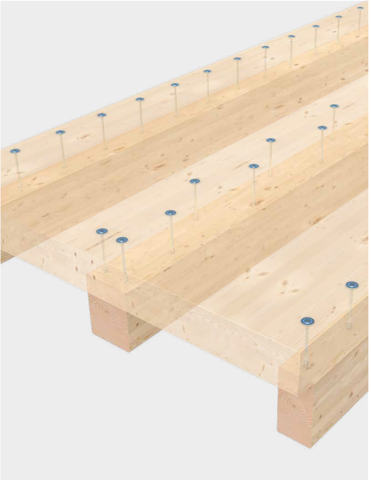
Bonding pressure distribution in the screw press bonding of rib panel elements
