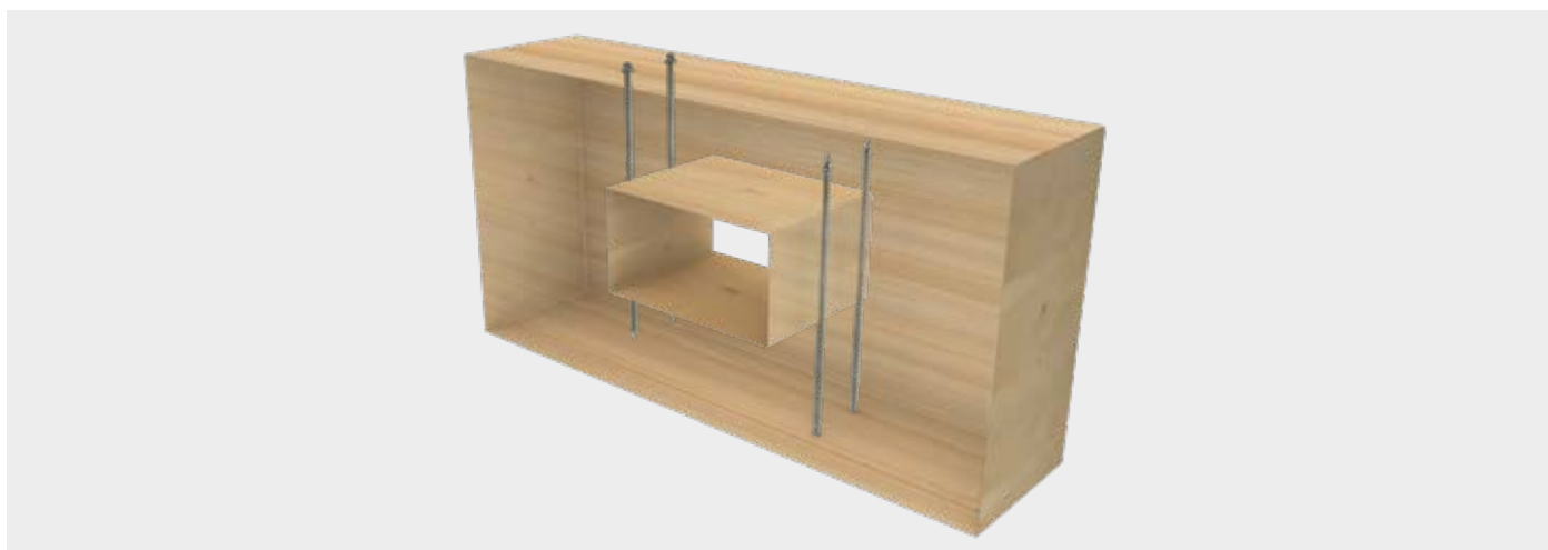
Reinforcement of beam openings
