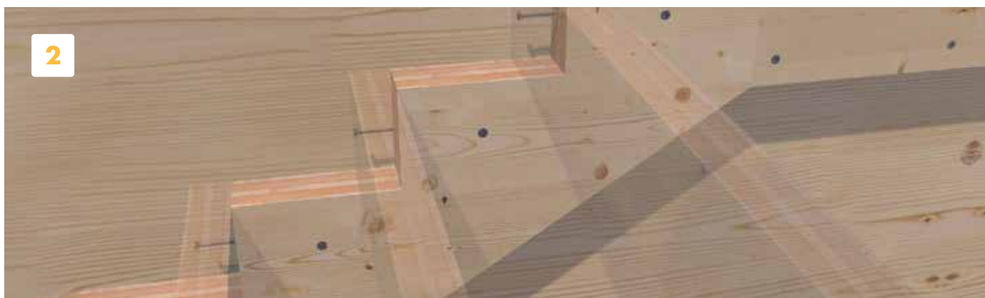
Attach the stringer to the front of the stair tread support using screws.
