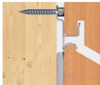
Wall connection with rhombus façade clip
