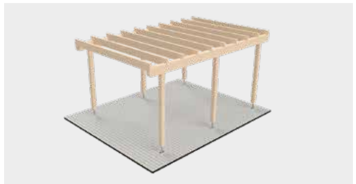
Design-based wood preservation in a carport with PediX Easy.
