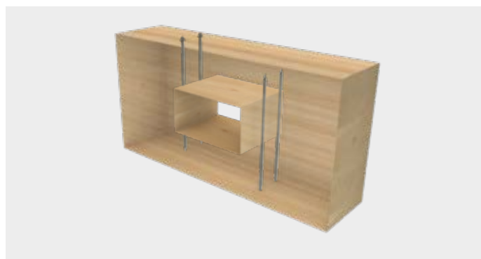
Reinforcement of beam openings
