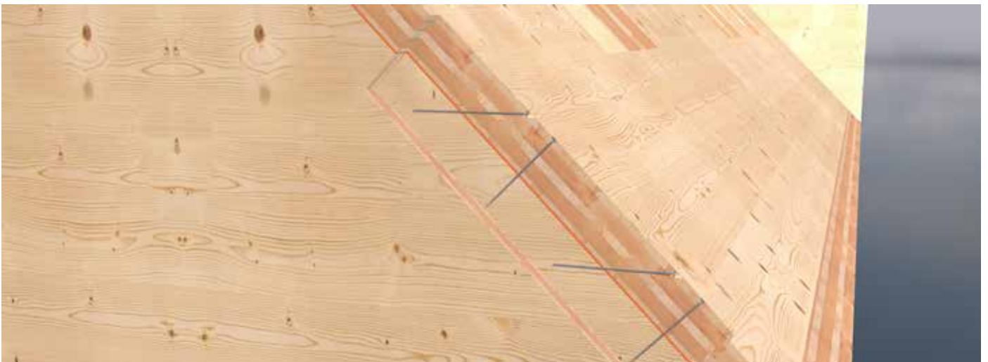
Connection of a roof and wall element
