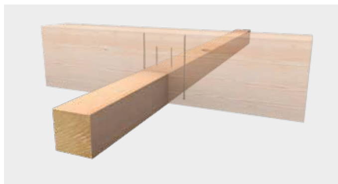
Reinforcement of the main/secondary beam supports
