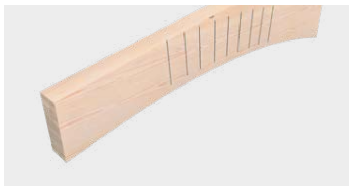
Reinforcement of trapezoidally shaped beams
