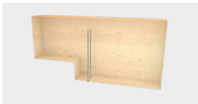
Reinforcement of notched beams
