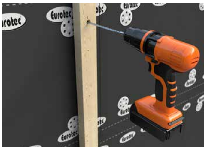
The support battens are placed on the insulation for installation. The masonry / concrete drill bit can be guided through the pre-drilled hole to pre-drill the insulation material and the substrate.
