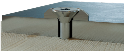
Countersunk head and rosette in a 90° hole
