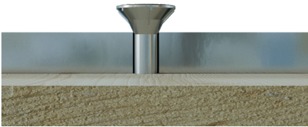
Countersunk head in a non-countersunk 90° hole
