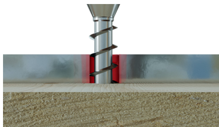
Thread damage caused by friction against the hole's wall
