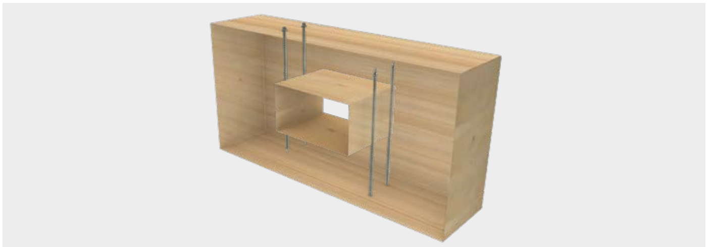
Reinforcement of beam openings
