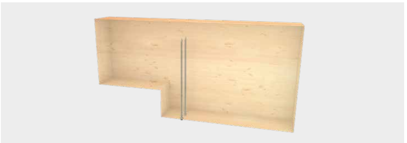
Reinforcement of notched beams
