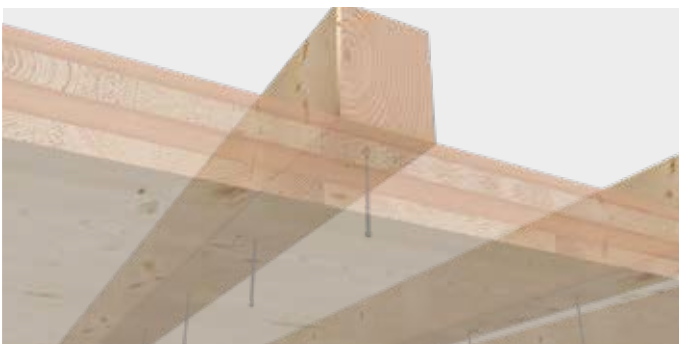
KonstruX DUO for the fastening of a covering
