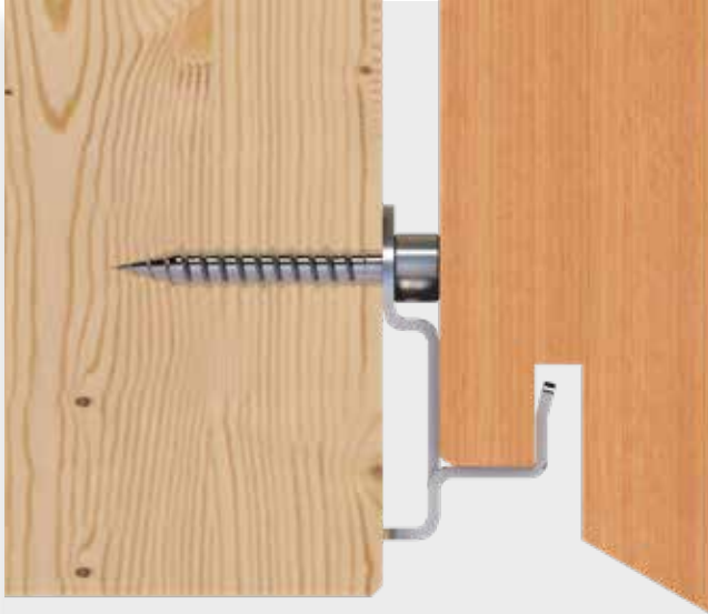
Facade clip for rhombus starter profiles used in a vertical timber sub-structure
