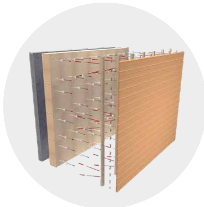
Facade structure with EiSYS-2s, exploded view
