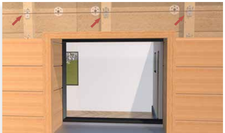
Facade profiles directly above windows and doors should also be fixed with an additional screw.
